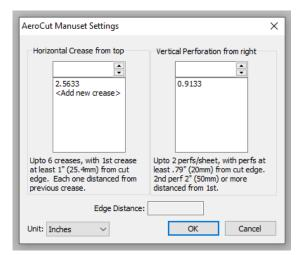
Creases and perforations are distances from the edge of the paper or the edge of the previous crease or perforation. You can also draw creases and perforations and then come to the configure menu (4) and make minor alterations to them.
